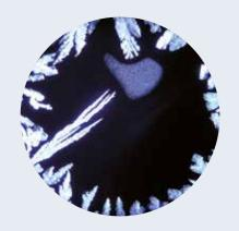
In this temperature range it is difficult to know, without visual observation, whether the system is controlling at the dew point, at the frost point, or somewhere in between. Since these states occur at different mirror temperatures for gas of the same water vapor content, it is important to determine which it is. Errors resulting from this problem can be up to 3°C.
