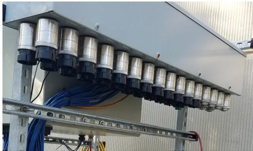
TruCal technology has been tested extensively to make sure that it performs under a variety of environmental conditions (see Fig. 3). The accuracy and T90 response times (shown in Fig. 4) have performed flawlessly even without calibration and with constant exposure to the elements. These sensors have been installed on the roof of MSA's manufacturing facility in Western Pennsylvania and exposed to all climates: hot, cold, rain, snow, sun, wind, humid and dry.
